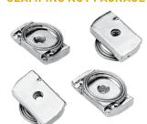
Twenty plated clamping nuts with top-grip nut retainers. Clamping nuts fit into mounting channels that are used on inside walls of Hoffman enclosures. Clamping nuts are included with all Hoffman accessories that attach to mounting channels. These clamping nuts can be used for mounting other equipment (brackets, etc.) to the enclosure walls.
